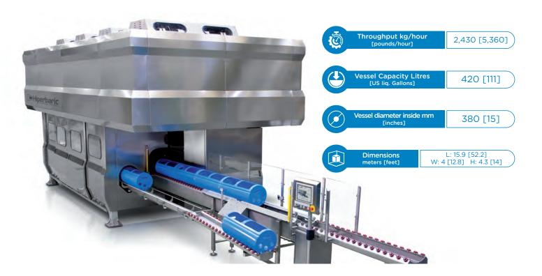
The Hiperbaric 420 is the best-selling HPP machines in the market. Its 420 liter capacity and 380 mm diameter vessel together with its 8 high pressure intensifiers allow this equipment to process more than 2 tons/h (4,500 lbs/h). This model is the first of our range with
